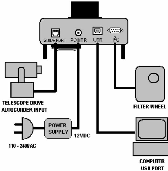
**GUIDE PORT:** This is where you connect the supplied 6 conductor modular phone style cable to the Autoguider (sometimes labeled "CCD") input port on your mount when using the STF-8300 as an autoguider, or when using Track & Accumulate with mount corrections (see the CCDOPS Manual for details of this mode)
