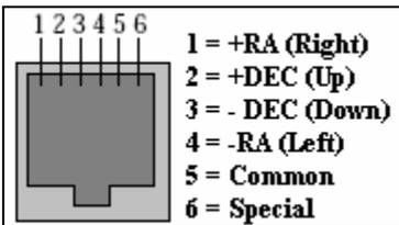
The *Left, Down, Up* and *Right* signals are driven from optically isolated photo transistors that conduct when telescope movement is desired. They can sink up to 25ma and can hold off up to 25V. If what you are plugging into is
