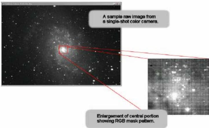
Single-Shot Color (SSC) cameras like the STF-8300C produce raw images that CCDOPS displays as monochrome until they are color processed. The Color Process command in the Single Shot Color menu of the Utility menu converts these raw images into color as shown in the dialog box shown below.
