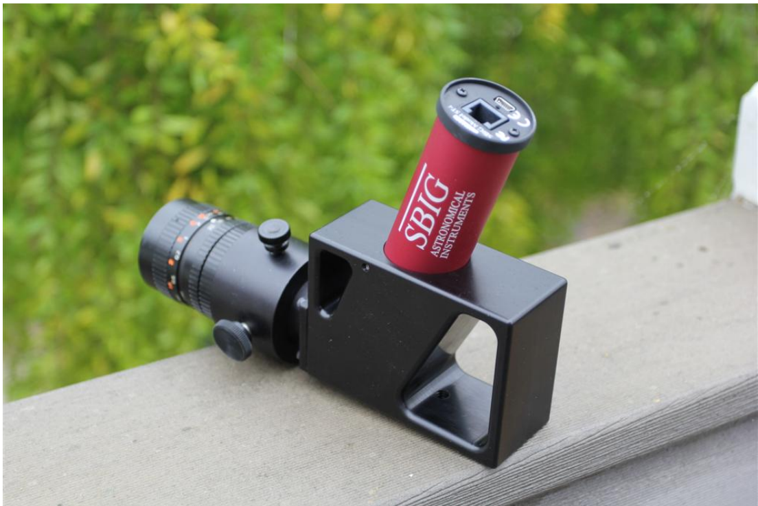
Figure Nine – C-Mount Lens Attachment for ST-I Spectrograph
