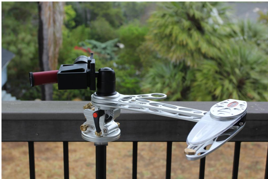
Figure Ten: AstroTrac Rotary Platform Turned Horizontal
