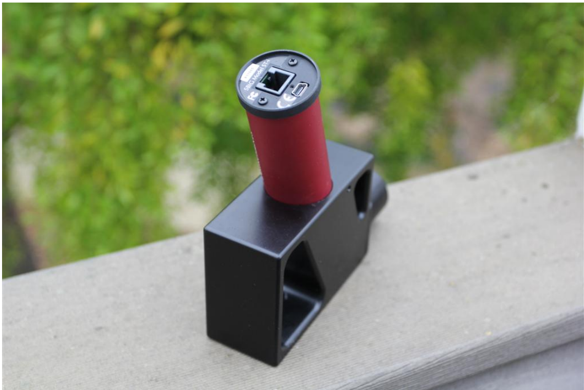
Figure Six: Correct Rotation Orientation of ST-i in the Spectrograph
