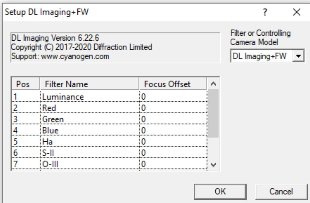
14. Click the Filter or Controlling Camera Model drop-down and select *DL Imaging+FW*. The default filter positions and names are displayed.
