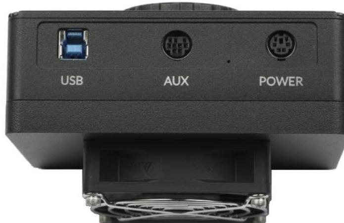
**USB** connector pinout is to the USB standard. The connector works with both USB 2.0 and USB 3.0 cables.
