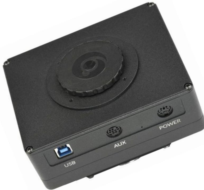
The STC-428-OEM scientific CMOS camera represents a major improvement over CCD technology. Compared with previous CCD models, the STC-428-OEM features higher sensitivity (78% QE versus 56%), significantly lower read noise (2.5 e- versus 9.3 e-), and 20X faster readout. While a single exposure can equal CCD dynamic range, the combination of fast readout and very low read noise allows for in-camera stacking using SBIG's StackPro™ to produce a greater dynamic range than previously possible.
