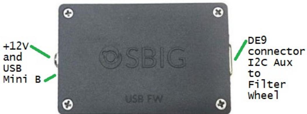
The 9-pin D-subminiature connector (sometimes called a DE9 or DB9) on the right side in the above photo is the connection to the SBIG filter wheel. It takes the place of the SBIG I2C AUX (Inter-Integrated Circuit Auxiliary) communication connection found on an SBIG camera. It provides power and control signals to the attached Filter Wheel.
