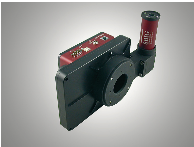
Fig. 1 Off-Axis Guider on ST-8300 and CFW-5
