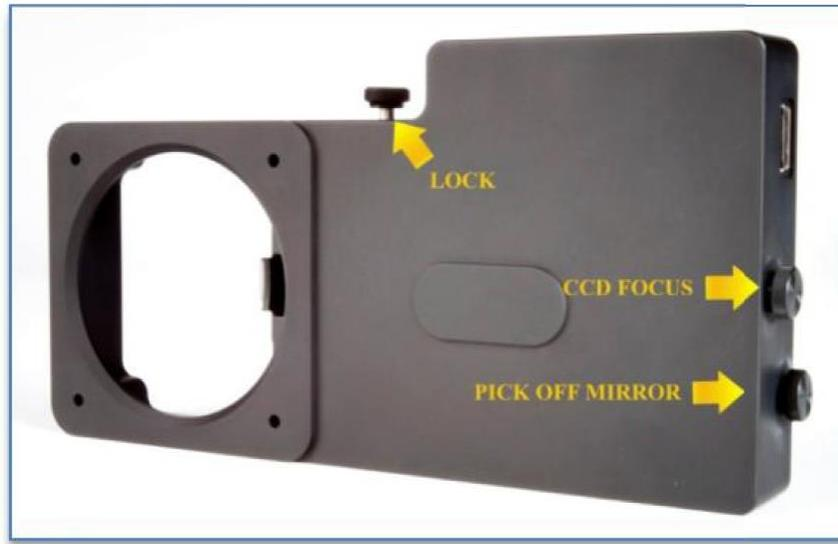
4. Locate the two adjustment knobs on the STX Guider used to set the placement of the pick-off mirror in the telescope's light path and to focus a guide star on the guider's CCD chip.
