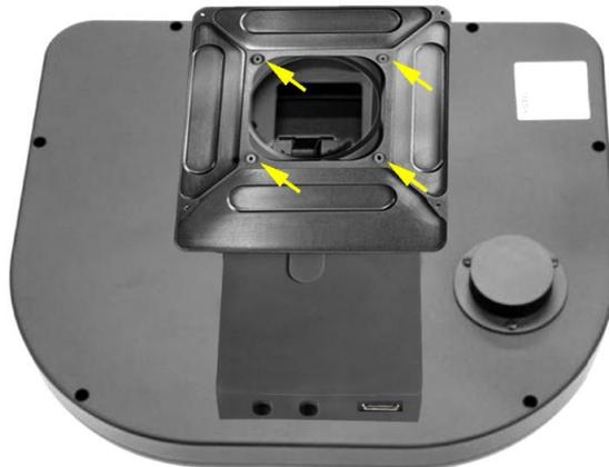
10. Place the AO-X body and front plate onto the rear plate and fasten them using the four screws removed in step 5.
