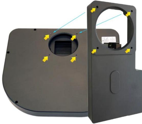
8. Place the AO-X rear plate on top of the STX Guider and align the four mounting holes.
