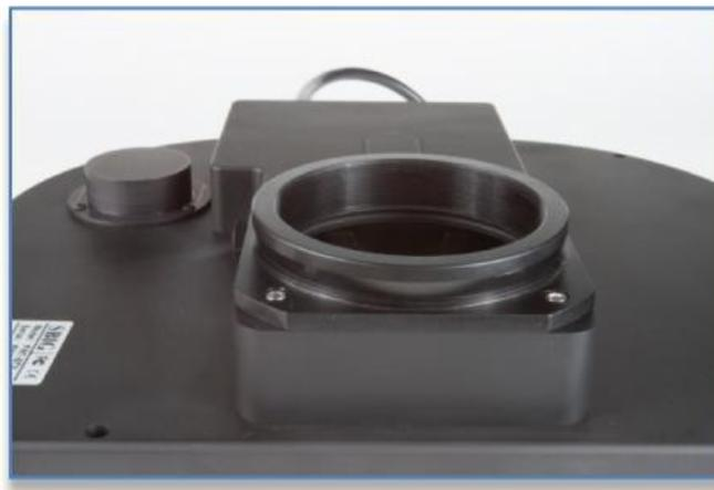
Thread and tighten the screws into the filter wheel.
