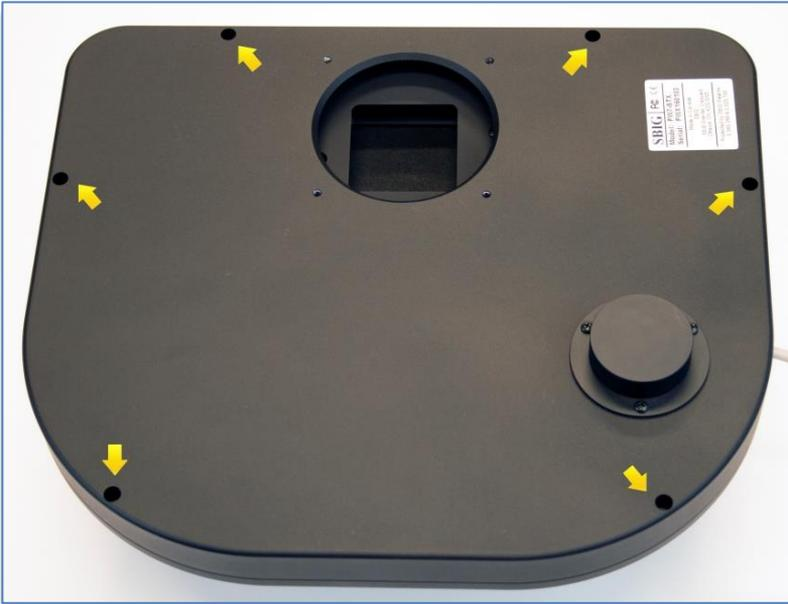
17: Attach the telescope coupling that you removed from the camera, with the shims in the appropriate locations. (The camera was supplied with a sheet indicating the shim positions.)
