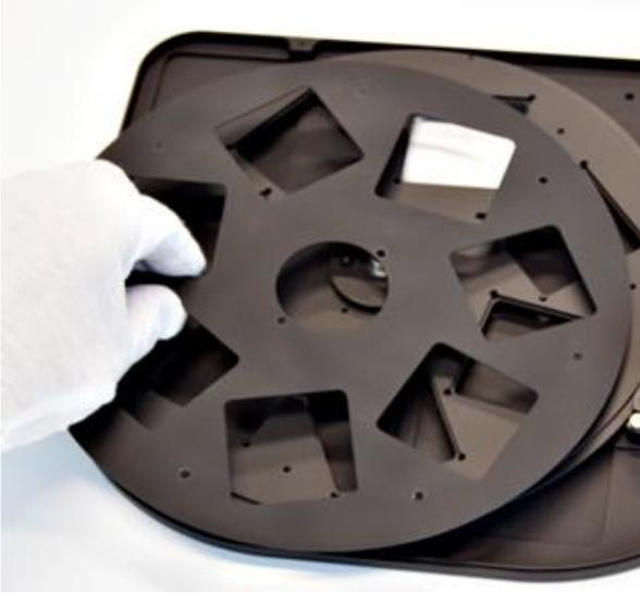
12: After press plate removal install each filter wearing clean cotton gloves
