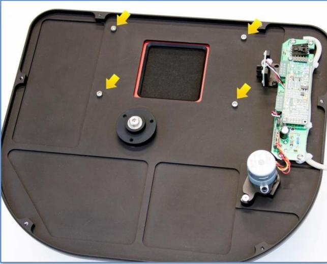
9: Reinstall the Carousel by aligning the bolt holes on the carousel relative to the bolt hole alignment on the spindle hub. Once the carousel has been inserted onto the hub insert the 3 cap head screws to secure the carousel.
