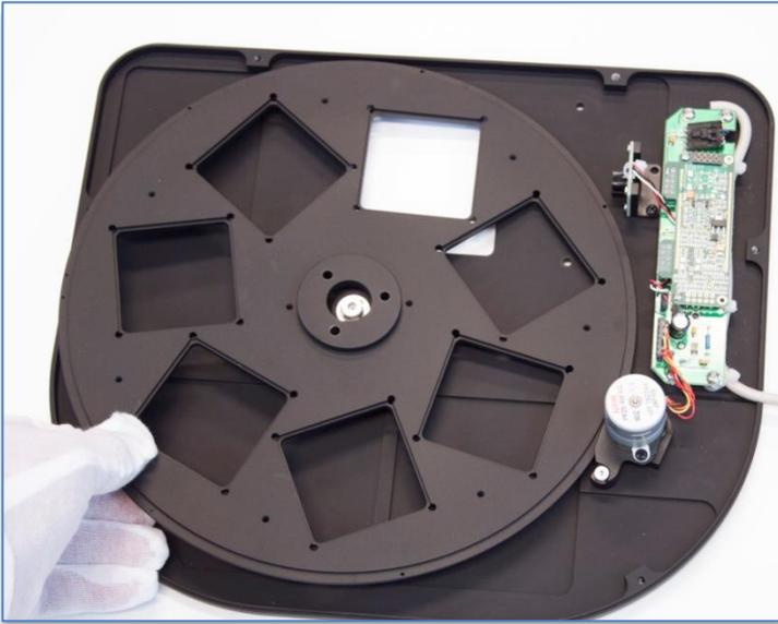
7: Align the filter wheel body holes with the outer holes of the camera.
