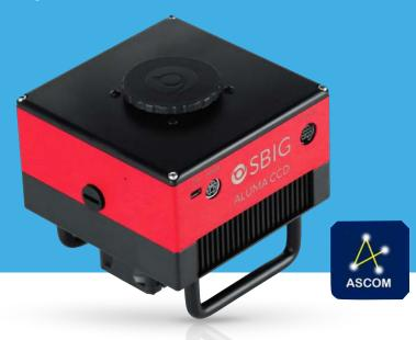
The SBIG ALUMA CCD cameras offer a choice of sensors allowing you to select the right pixel size and imaging array to match your application and budget. Sensor options range from from 1-megapixel to 9.1-megapixel arrays from 24µm to 3.69µm square pixels. Peak quantum efficiency (QE) ranges from 75 to 93%.
